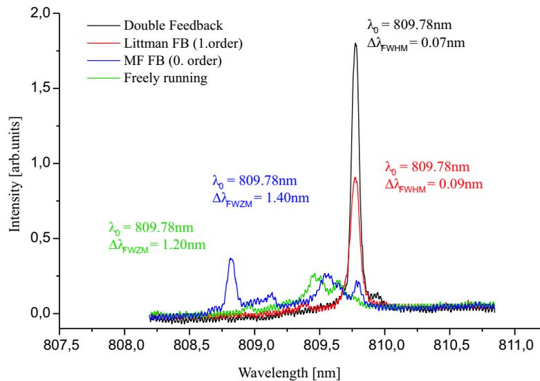
Fig. 3. Spectrum of the double and single feedback laser. Black spectrum: Double feedback applied; Red spectrum: Feedback from first order applied; Blue spectrum: Feedback from zeroth order applied; Green spectrum: Freely running laser.
