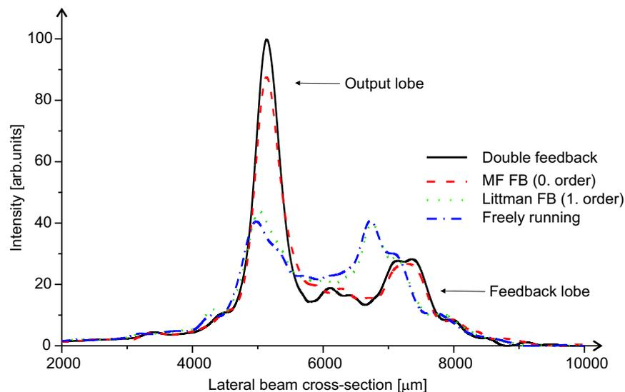
Fig. 2. Intensity profiles in the lateral far field of the double feedback (solid), the single feedback (dashed and dotted, respectively), and the freely running (dash-dotted) BAL.
