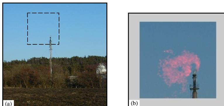
Fig. 2. (a) Flare LT1 at the polyethene plant. (b) (2.0 MB) Movie of ethene gas cloud escaping from flare LT1 as visualized with the system ([6.0 MB version](#)).
