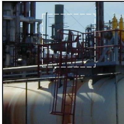
Fig. 6. (1.6 MB) Movie of ethene leakage. By sweeping the camera system over the polyethene plant, a leakage was found. A visible image and a sequence of gas images are shown. The gas-correlated images are merged with the zoomed visible image. The ethene gas leakage was taken care of immediately by the operating personnel ([3.8 MB version](#)).
