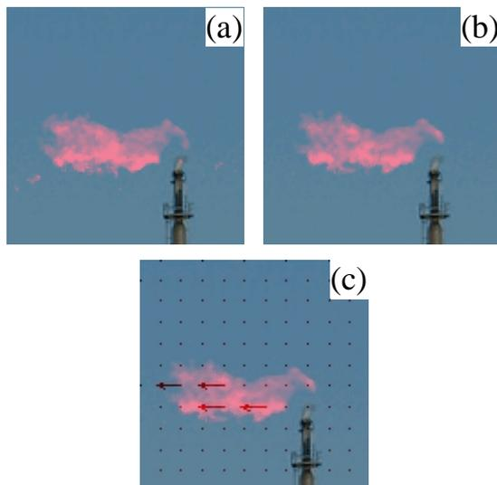
Fig. 11. (a) Gas-correlated ethene image at time  $T_0$ . (b) Gas-correlated ethene image at time  $T_1$ . (c) Wind vector map derived by cross-correlating the gas-correlated images at time  $T_0$  and  $T_1$ . The resolution of the vector map is determined by the size of the small cross-correlation matrixes.
