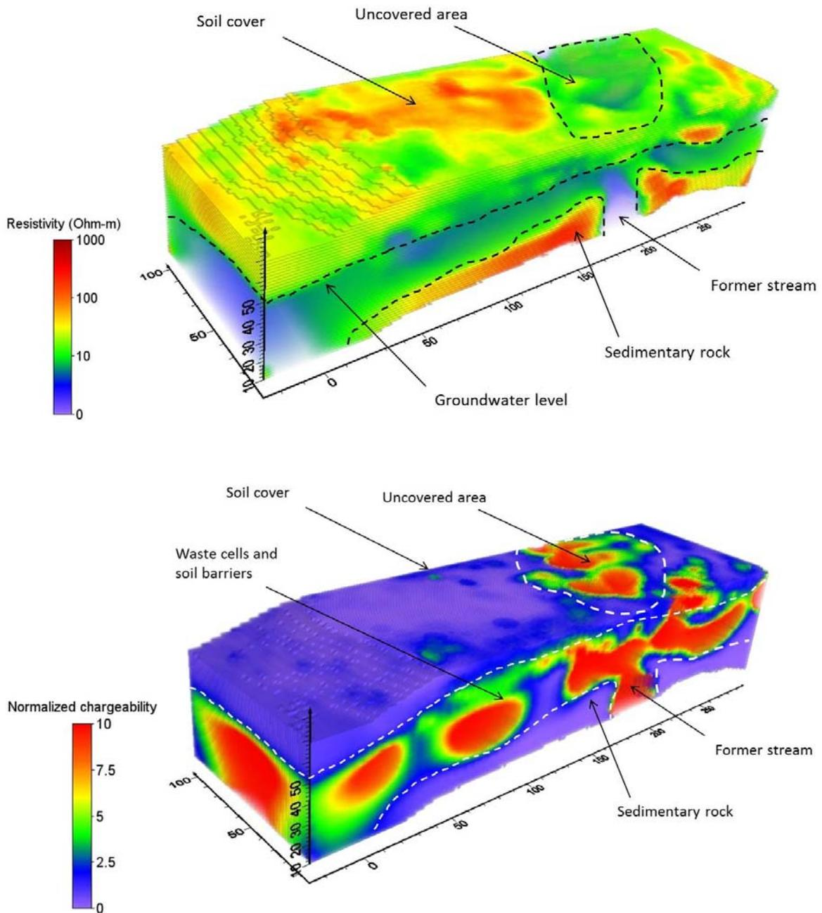
Figure 3. Example result from the MaLaGa-project - Large scale model based on resistivity and IP data from the Filborna landfill site, Helsingborg, Sweden.
