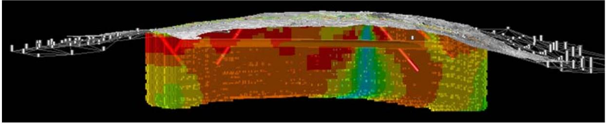
*Figure 2. 3D model of the rock resistivity along a road tunnel, with tunnel and borehole positions shown. The low resistive zone probably means fractured and weathered or water bearing rock. Since the drilling was done before the geophysics the zone was missed.*
